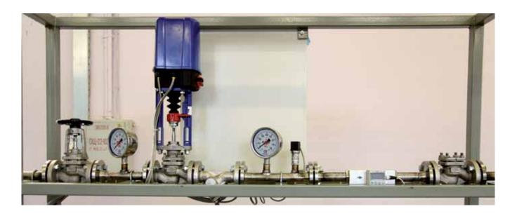
Units for pulsation and barbotage of flushing water are additional devices for flushing stands, strictly required when manufacturing complicated marine engineering articles, assembly of systems, and can be used as well when flushing systems with standard pumps.
